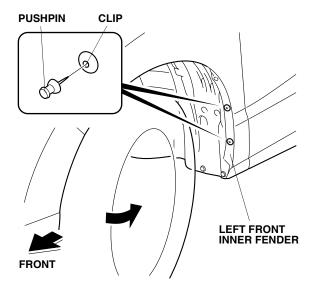
3. Remove two self-tapping screws from the left front inner fenderwell.
