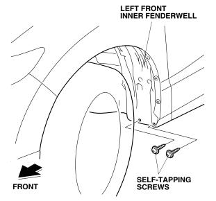
4. Install the left front splash guard to the left front inner fender with two washer-screws and the two self-tapping screws removed in step 3. Tighten in the order 1→2→3→4.
